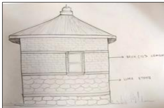
Fig. 12 (c): Modern Bhunga with brick and stone construction
