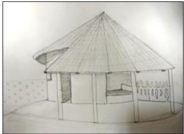
Fig. 12 (b): Bhunga house having roof supported by precast columns and addition of seating areas
