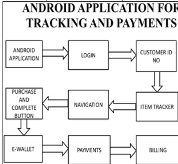
We are using android application in the purpose of tracking and payments. Android application having a login page for user and admin. For purchasing customer need to register with customer ID number. Then customer need to add list of product then it automatically navigated.
