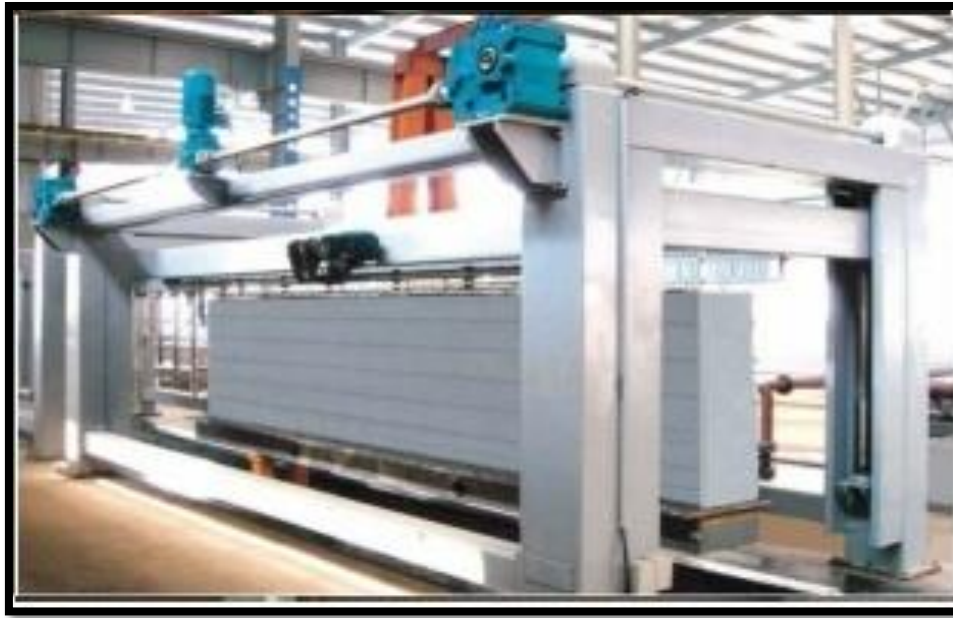
Fig. 6: Cutting process of AAC Block
