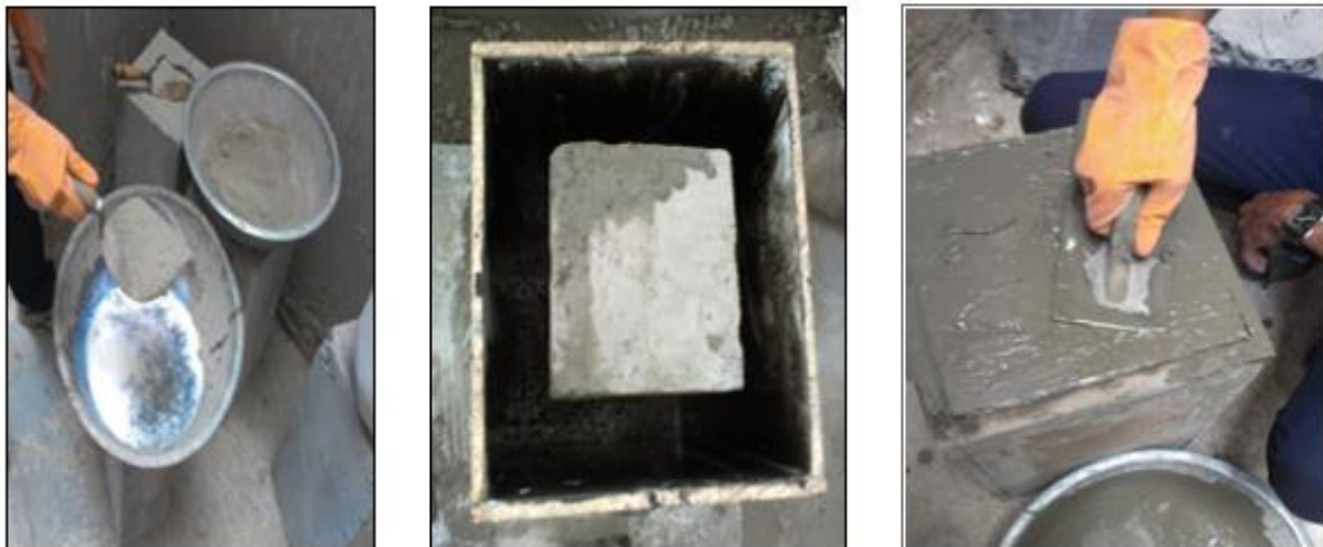
Fig. 3: Application of SBR on specimen_SK and Finishing
