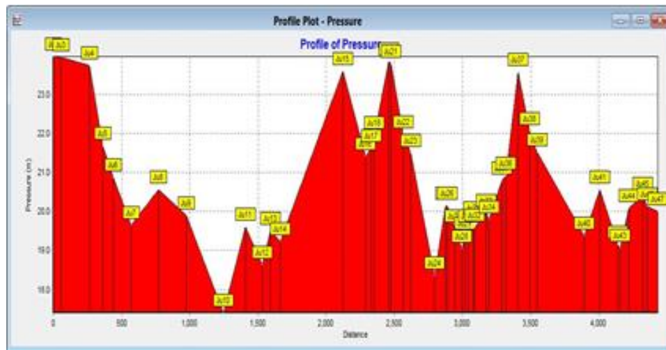
Fig. 9: Pressure Profile of WDS ESR E10
