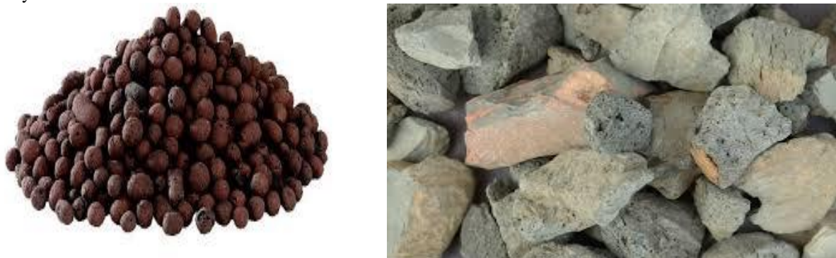
Fig. 11 & 12: Light weight aggregate: “Aggregate that is clean, green and lean”
