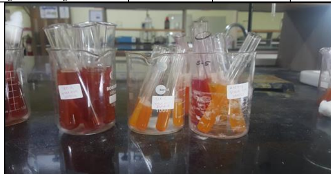
Fig. 5.14: Tap water + 0.5 ml sewage + 3 g/l cow dung ash ( 6 hrs contact time )
