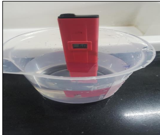
Fig. 3: pH measurement by using Pen probe type pH meter
