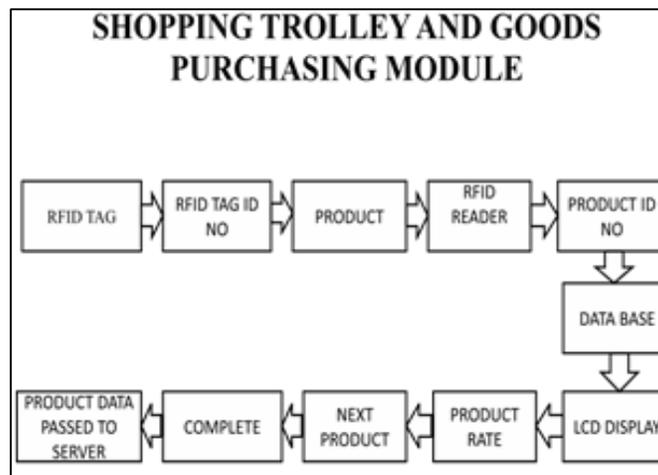
In this module shopping trolley contain particular RFID tag and it can be read by RFID reader. When the customer put the product on the cart all the details are readed by RFID reader and displayed on the LCD. Product data passed to server through NRF module.
